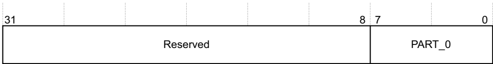
Figure 3-23 STMPIDR0 bit assignments
